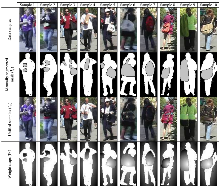
Fig. 3 Data samples from the VIPeR database, their corresponding segmented image I_s , the unified samples, and the proposed weight map ( W )
