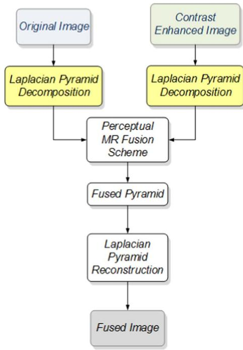
Fig. 1. Block Diagram of the Fusion Methodology.
