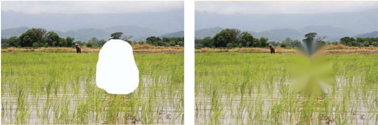
Fig. 9. An example of blurring artifacts in PDE-based image inpainting method, original image with large hole to be filled (left), inpainted image using [12,2] with introduced blur into the large restored regions (right).
