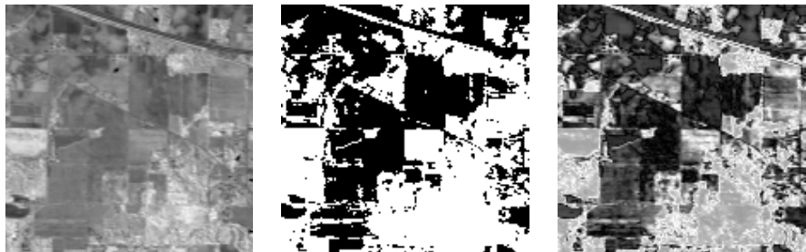
Figure 5: Left: Original bandwidth intensity image. Center: Thresholding with crisp assignments. Right: Thresholding with soft assignment.
