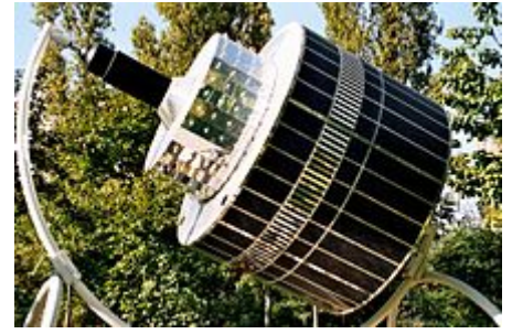
Model of a first generation Meteosat geostationary satellite.
