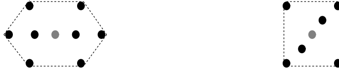
Fig. 6.2. The clusters, formed by the black points, can be represented by their codevectors (grey points). Dashed polygons identify the Voronoi sets associated with each codevector.
