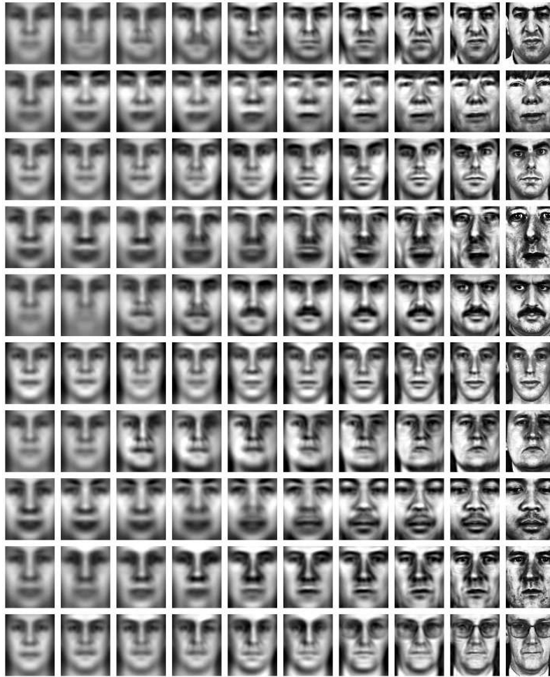
Fig. 13.5. Reconstruction. Each row shows how a face image is reconstructed using an increasing number of eigenvectors. The first image (starting from the left) uses 10 eigenvectors; the second uses 20 eigenvectors; and so on. The last image of each row is the original picture.
