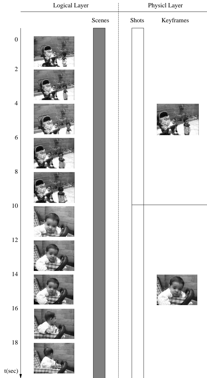
Fig. 14.1. Video structure. The picture shows the main components of a video.
