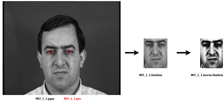
Fig. 13.2. Face localization. The picture shows how the face is first localized and then normalized out of the original image (courtesy of Sébastien Marcel).
