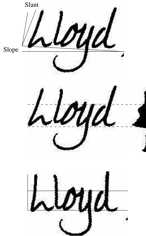
Fig. 12.2. Handwritten word normalization. The upper picture shows slant and slope, the central picture shows the so-called core region (the region containing the character bodies), and the lower picture shows the result of the normalization.
